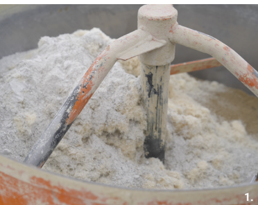
1. Mixing 3D printing materials
