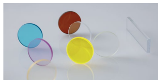
Examples of various colors by changing dopant ions in YAG
