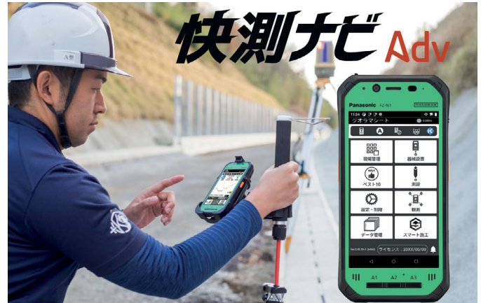
Enabling single-person measurements with integrated surveying equipment
