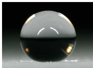
Fig. 1: Ball-shape droplets form on HIREC surface
