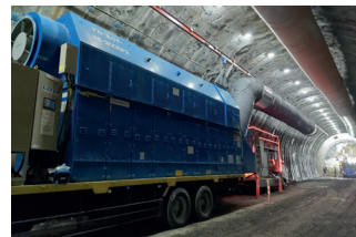
Large dust collector (3,000 m 3 /min)
