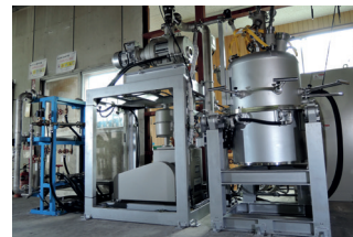
30kg vacuum induction furnace for R&D melting
