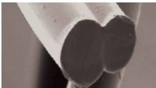
Cross section of LYCRA® T400® fiber
