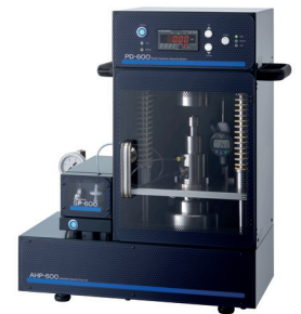
Automatic Powder Resistivity Analyzer MCP-PD600 for Li-ion battery market
