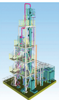
3D model of ammonia stripping facility
