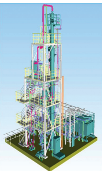
3D model of ammonia stripping facility
