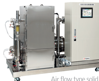
Air flow type solid state fermenter for laboratory use
