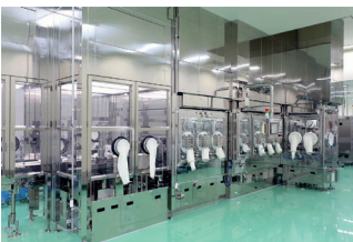
Aseptic/hazardous filling system for anti-cancer drug
