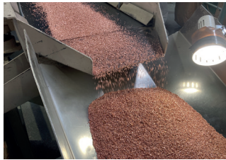
Metal recycling (copper sorted from coated wire copper)
