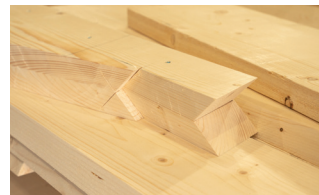
Precut roof parts
