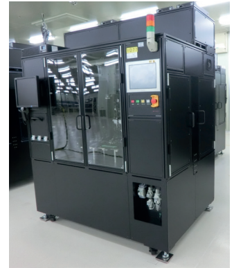
Fully automatic tester for camera module
