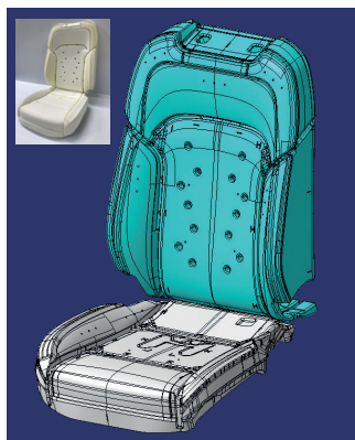
Seat pad and CAD drawing
