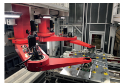
D-MAT: Press-to-Press Transfer System
