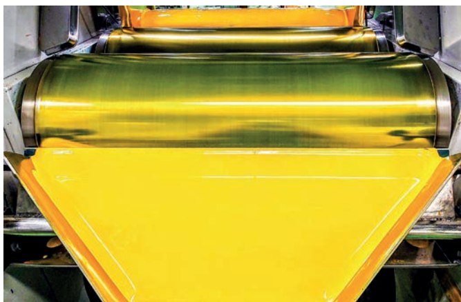
Ink production by three-roll mill
