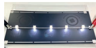
Conductive ink as substitute for wire harnesses
