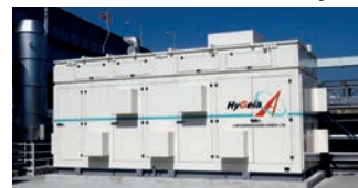
HyGeia-A: small-scale on-site hydrogen generator
