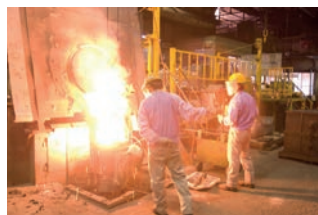
Melting raw materials in a high-frequency electric furnace
