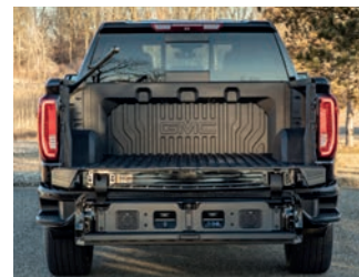
Sereebo® carbon fiber reinforced thermoplastic, as used in the GMC Sierra Denali 1500
