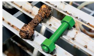
After a 2000-hour Salt Spray Test: TAKECOAT®-1000 (right), Electro-Galvanized (left)
