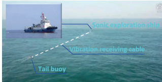
Sonic exploration using a ship
