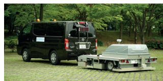
Vehicle-towed ground penetrating radar exploration vehicle
