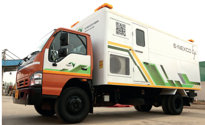
Network Survey Vehicle "E-NEXCO Eye"
