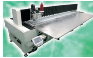
Large-scale sewing machine (2500 x 700 mm)
