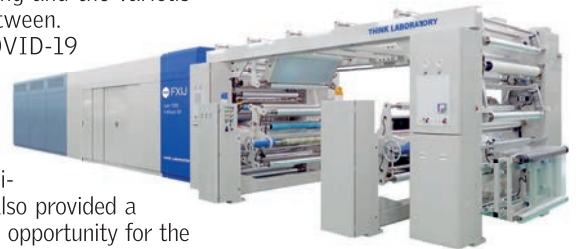
FXIJ type 1000 FullAuto SP Inkjet Printer with water-based ink
