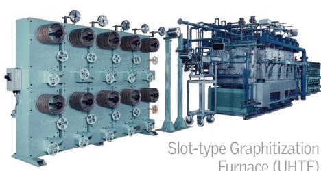
Slot-type Graphitization Furnace (UHTF)
