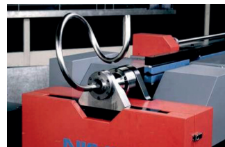
Nissin CNC Freeform Tube Bender (NFB) to which die making technology is applied
