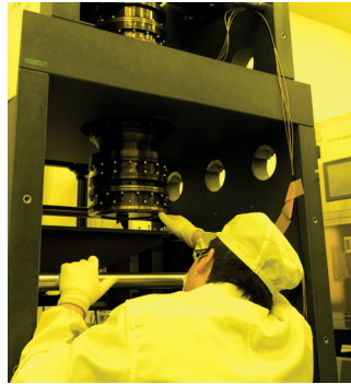
Assembly and adjustment of Projection Exposure Lenses
